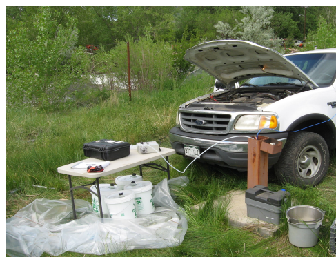
Conducting pump test at CSMRI-8 and recording water level data to determine hydraulic conductivity.
