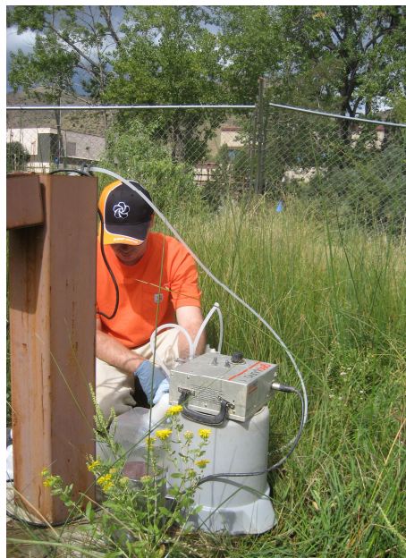
Groundwater sampling using peristaltic pump.
