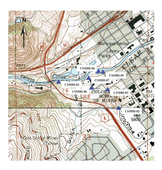
Figure 3-6 Locations of Ground-Water Monitoring Wells
